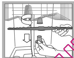
To remove the upper sprayer arm, rotate the locking ring in an anti-clockwise direction.
