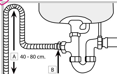
The outlet hose must be at a height ranging from 40 to 80 cm from the floor / surface where the dishwasher rests (A). Before connecting the water outlet hose to the sink drain, remove the plastic plug (B).
