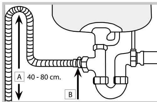
The outlet hose must be at a height ranging from 40 to 80 cm from the floor / surface where the dishwasher rests (A).
